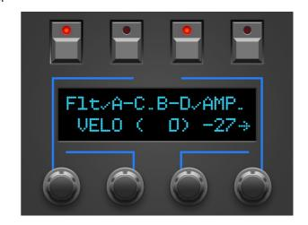
Line 2 also indicates the slotname (LFO1, PRESSURE ....) as well as the current modulation depth; as usual the program's original value in brackets and the currently set/edited value afterwards.
