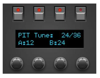
As already mentioned, the Relative mode only makes sense if Edit A <u>and</u> B are both on. 'Relative' will be deactivated as soon as only one of the Edit buttons is active. At the moment you activate both channels again, the lastly selected state (on or off) for Relative will be resumed again.
