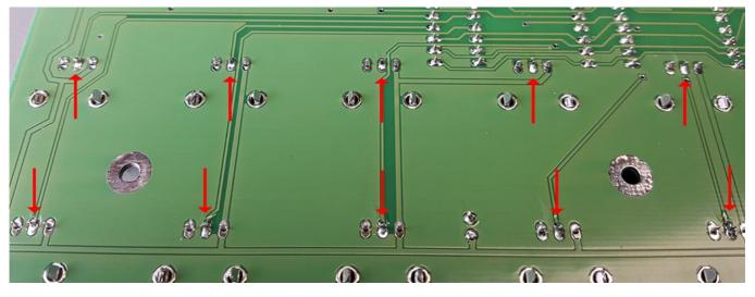
Now they are kind of fixed althoug they still can tilt a bit. Now you can examine all pots once again, maybe one got tilted by putting the PCB on the table. If one must be corrected you simply can do that by just heating up this middle pin.
