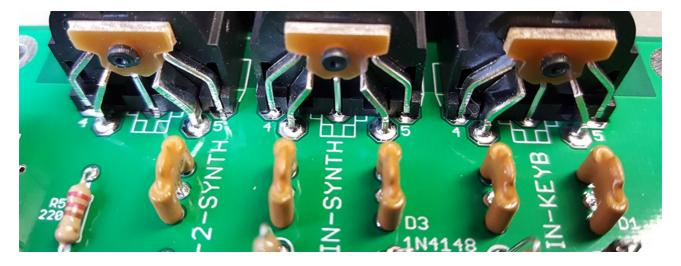
Solder all remaining pins and do not be stingy with tin and time. If the pin and the leg are heated up properly and you give the tin a bit time to flow, it will crawl through the via onto the other side of the PCB as the picture above shows quite well. That's what we want - the jack will be stressed mechanically later by midi cabled being pushed in and ripped out.
