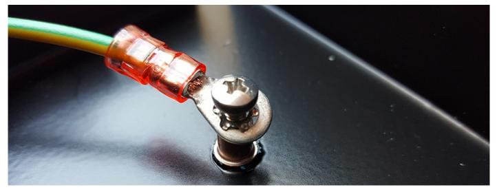
The ESD-cable screw of the upper case is a bit more difficult as the opposing case wall is in the way when trying to use a screwdriver. It's easier to fix it with a pliers as shown in the picture.
