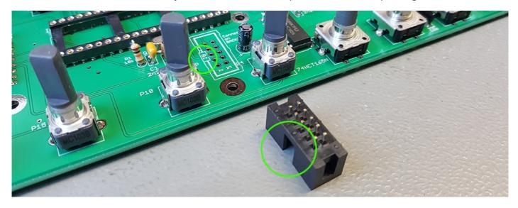
The connector for the display is pointing to the right side:
