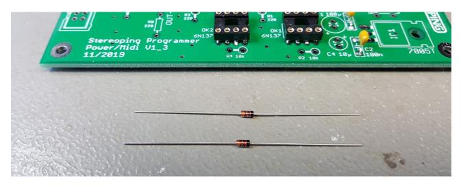
Now on to the two diodes. They have a black mark on one side. This mark can also be found on the PCB and should match the mark on the diode. Well, the mark for the red diodes unfortunately can hardly be seen on the silkscreen. Looking onto the PCB with the type 'Stereoping Programmer, Power-Midi V1\_3' to the left bottom, the mark of the red diodes must point to the RIGHT – like they are already layed out on the picture above.
