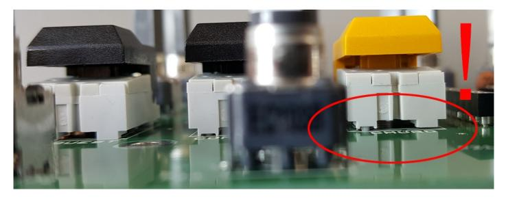
After the buttons you can push the LEDs into position. **Attention – mind the polarity!** To the left of the button near the LED you find a little '+', this is the side for the longer LED leg to go.
