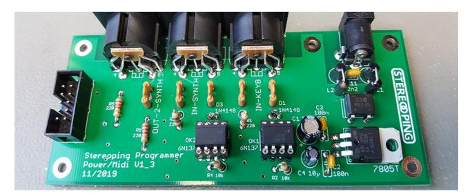
One little word: if you got the PCB laying in front of you like on the picture above, the optocouplers will be plugged into the sockets upside down. Therefore another detail picture:
