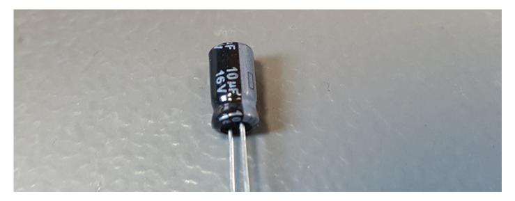
You already know the smaller  $10\mu$ F cap from the power midi board. This is for position C6, mind the polarity! Long leg into the pad where the small + is in the silkscreen.
