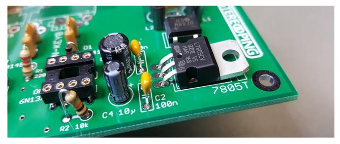
The regulator pulls the legs a bit out of the PCB automatically, that's ok. Now you can solder it from the backside. Take care to make clean soldering marks. Especially the middle pin is important. The goal is not to use much solder tin, but to make a clean and proper soldermark.
