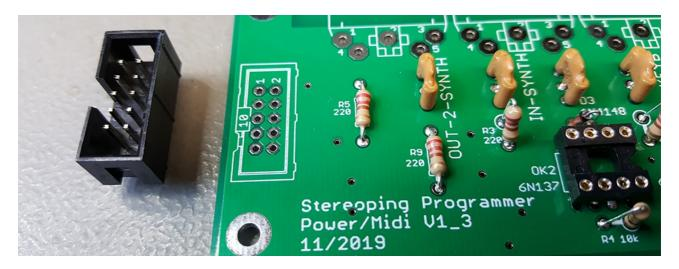
Place the connector from above – **take care for the right direction of the cavity!** It should be on the same side as the silkscreen shows. We recommend soldering one leg first and check again for the connector to sit flat on the PCB. Then the other legs can be soldered. Take your time (4-5 seconds per leg) to allow the tin to flow through the via onto the other side of the pad.
