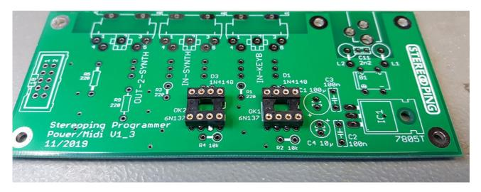
The notch indicates where to put leg Nr. 1 of the IC – leg 1 is indicated by a notch in the case or a point printed together with the device name. Putting an IC into the socket the wrong way sometimes (not always) can damage the part. There is no reason to worry here for the optocouplers.
