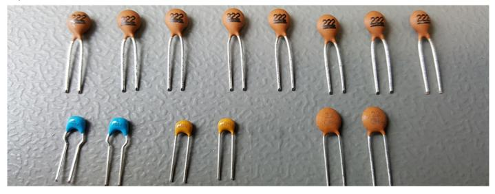
Ceramic capacitors do not have polarity. Place them as you like, bend the legs a bit, solder them and cut off the wires. Their real color and look might be different than shown on the picture above! There are 4 different values:
