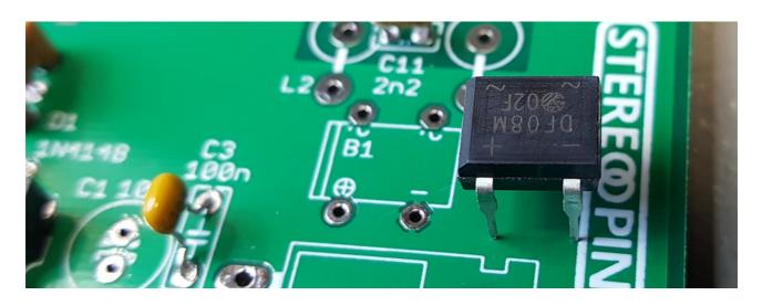
There is a second aid: one edge of the rectifier is sloped (yellow arrow), the PCB got as double line on this side (green arrow).
