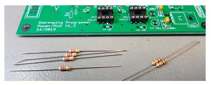
Resistors also do not have any polarity, place them as you like. As all parts, they should be soldered as narrow to the PCB as possible. To fit their solder pins one leg must be bent 180 degrees. On the solderside bend the legs away from each other to prevent them slipping out of their holes when turning the PCBs. After soldering cut off the legs and we're done here.
